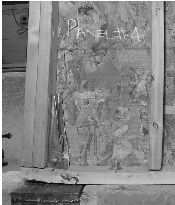
Figure 5.6. Failure components panel 4.
